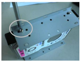
Figure 5: Attach the HDD to the bracket
